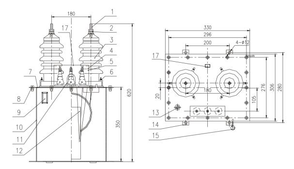
1.Conducting rod 2.Standard piece 3.Primary porcelain bushing 4.Conducting rod 5.Standard piece 6.Fixing bushing 7.Cover 8.Standard piece 9.Oil indicator 10.CT body 11.Secondary porcelain bushing 12.Iron core and coil 13.Oiling hole 14.Mounting base 15.Breather 16.Name Plate 17.Sealing cover
